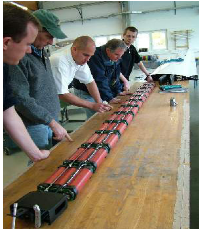
A massive array of batteries are stored in the Antares' wings.
